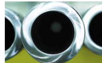
Our drill pipe assembly line at Mongstad offers new 5" and 5 1/2" Drill pipes are manufactured to API specification 7.
