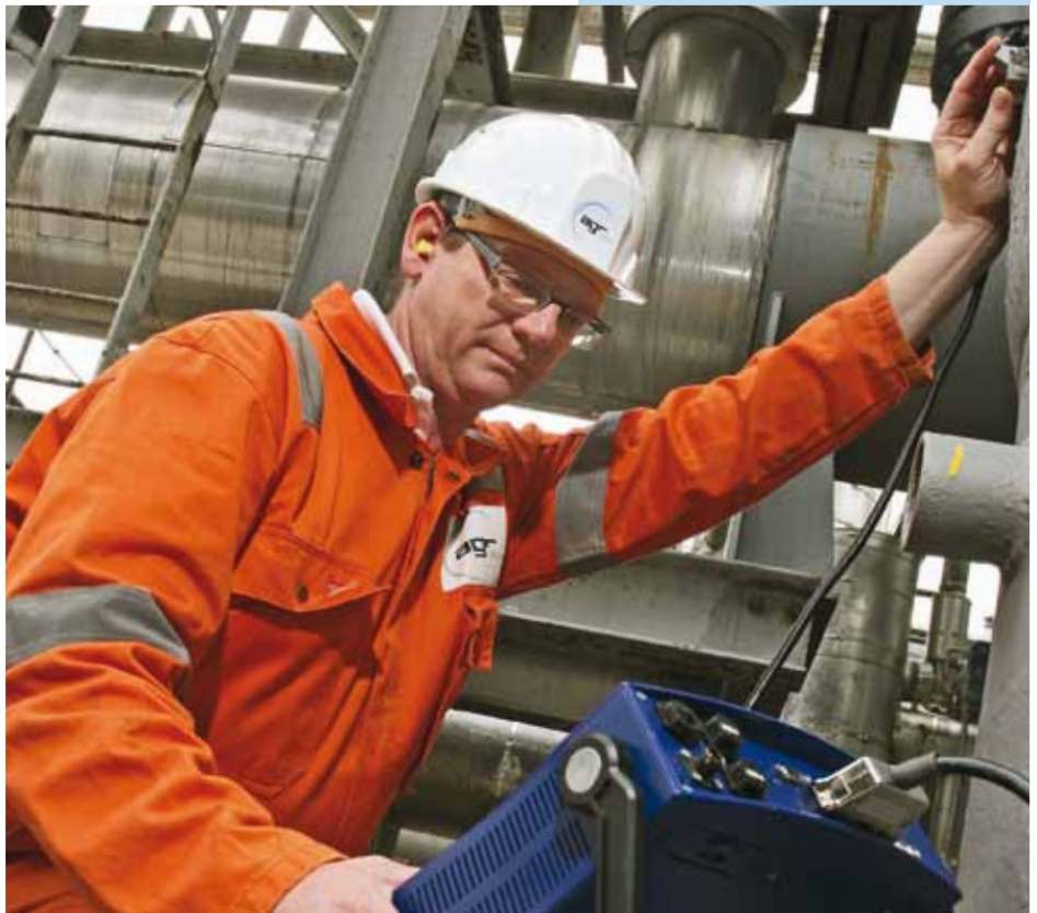
Ultrasonic inspection using TD Handy-Scan®
