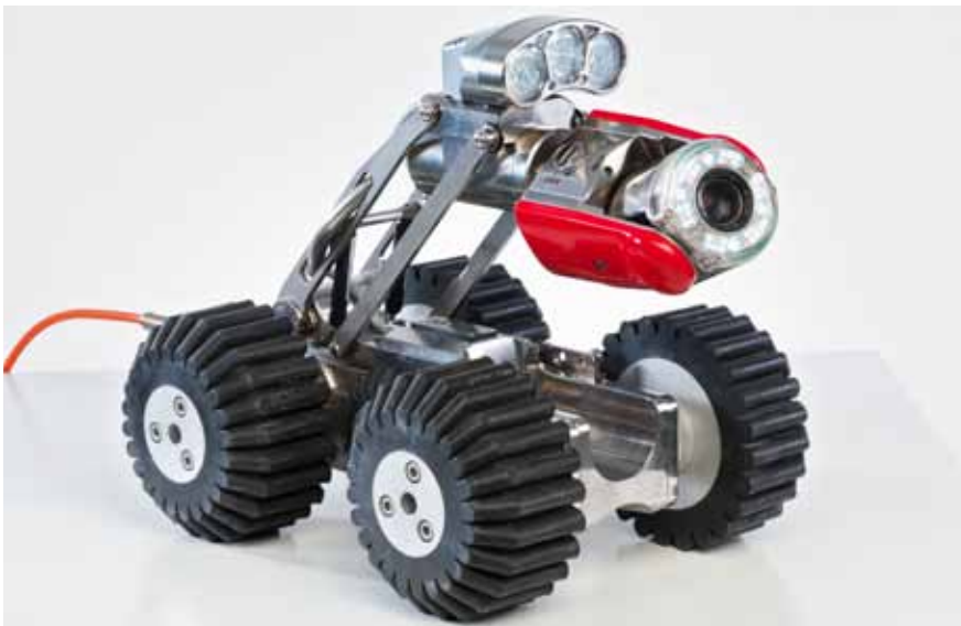
Typical Inspection Camera with Crawler
